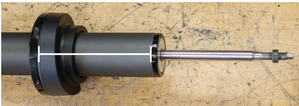
Fig. 14: Measure from the preload ring to the bearing cap.
