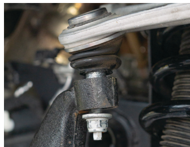
Fig. 5: Separate the UCA from the upright.
